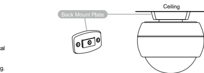
5. If using the Back-Mount Arm, utilize one 3x10mm screw to attach the Back-Mount Plate to the Back-Mount Arm. Then affix the Back-Mount Arm to a surface utilizing the provided 3x20mm screws.
