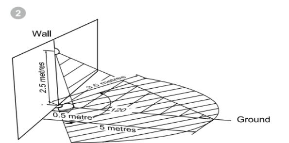
Further, for optimal performance your MultiSensor should NOT be mounted directly on or near metal framing or other large metallic objects. Large metal objects may weaken the Z-Wave wireless signal.
